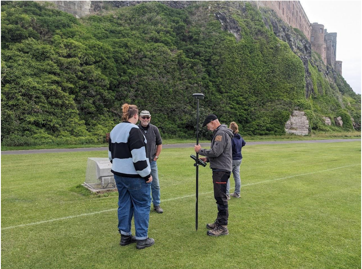
Figure 15: Volunteers from the Bamburgh Research Project using the GPS to establish a survey grid in the Cricket Ground (photo: K. Strutt)
