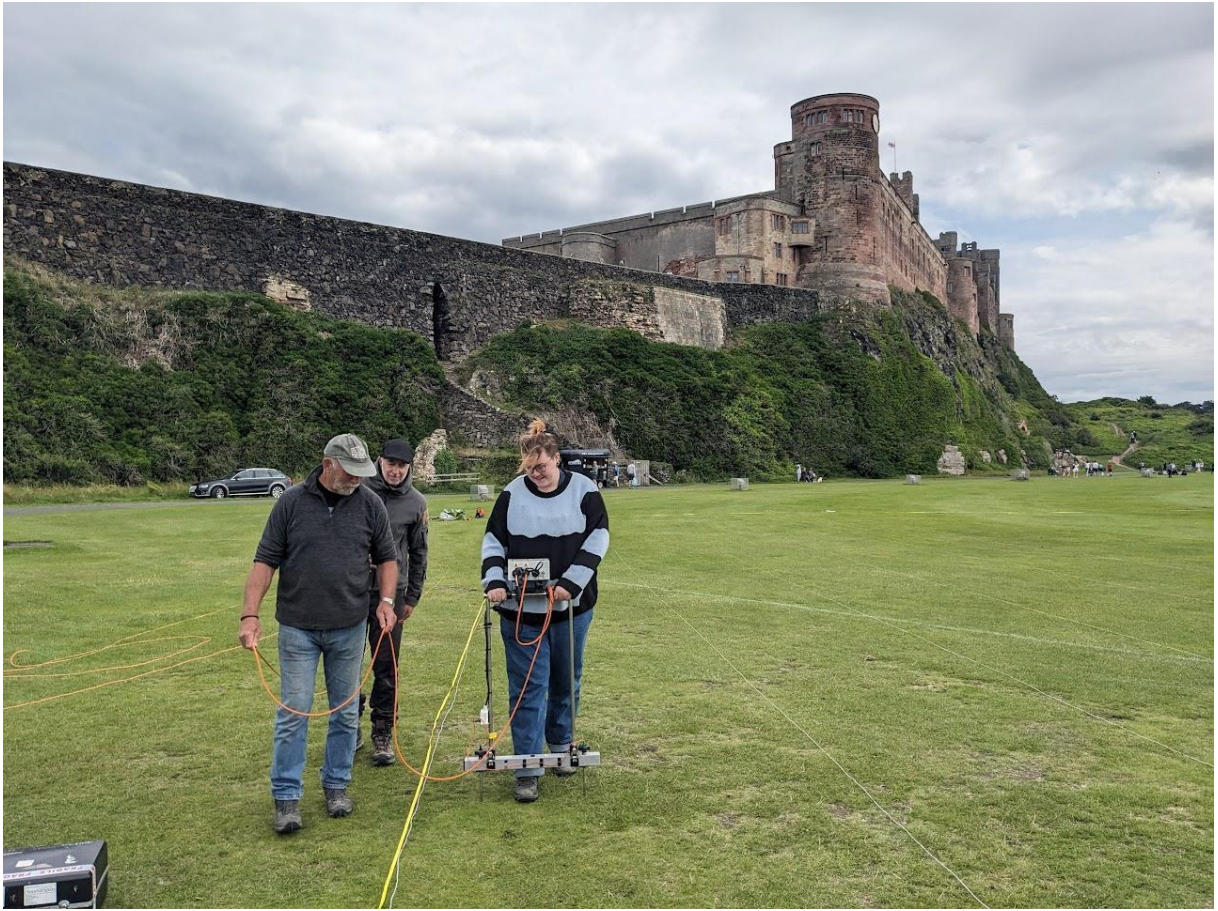
Figure 17: Earth resistance survey being carried out by BRP volunteers (photo: K. Strutt)
