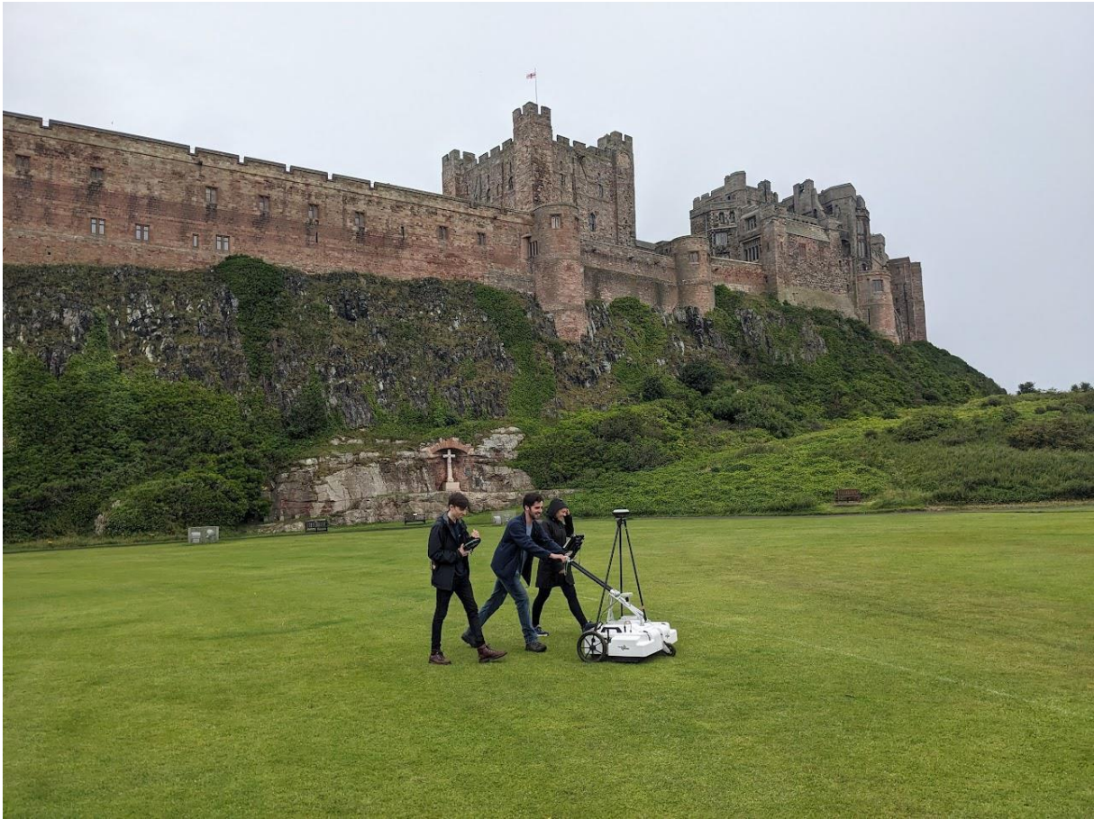
Figure 18: GPR survey under way across the Cricket Ground using an Impulse Raptor 8-channel system and GPS (photo: K. Strutt)
