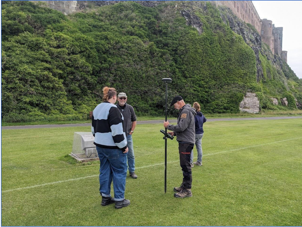
Figure 7. Volunteers from the Bamburgh Research Project using the GPS to establish a survey grid in the Cricket Ground (photo: K. Strutt)
