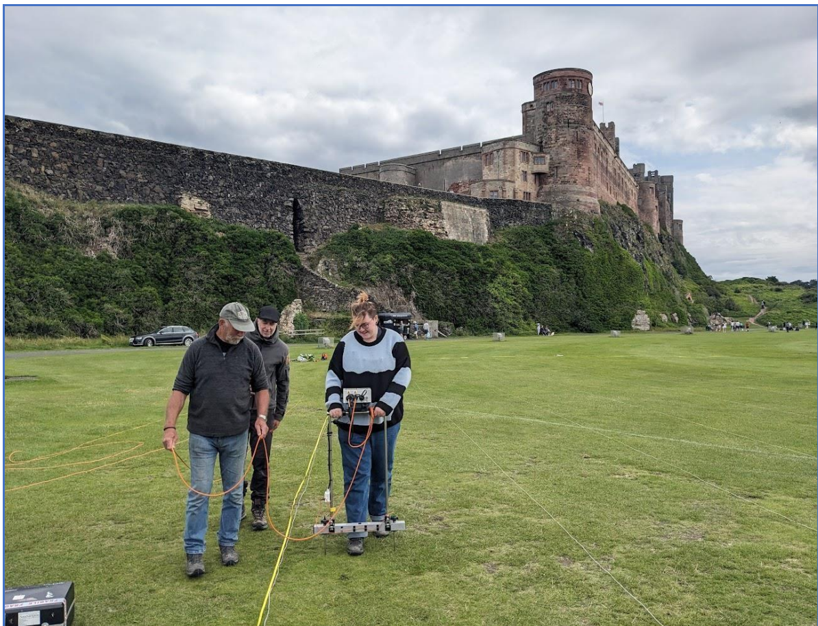
Figure 9. Earth resistance survey being carried out by BRP volunteers (photo: K. Strutt)
