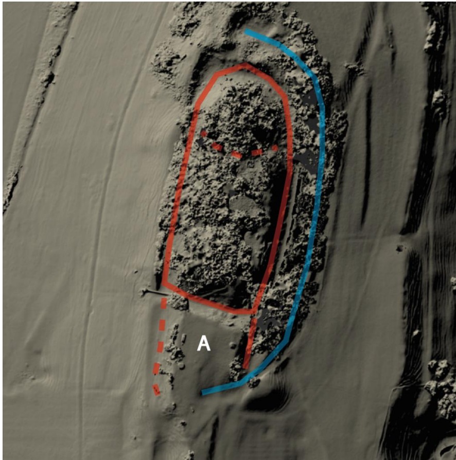
Figure 6. An interpretive scheme of the castle layout, with the motte defined at the top of the complex, the inner bailey in the centre and the outer bailey at the bottom (A). This simple delineation would suggest that the outer bailey came into existence with the cutting of the second, outer ditch on the north side of the castle (shown in blue), but the evidence is so distorted that it is feasible that the outer bailey was an original feature of the first castle constructed on the site (original model by Adam Stanford).
