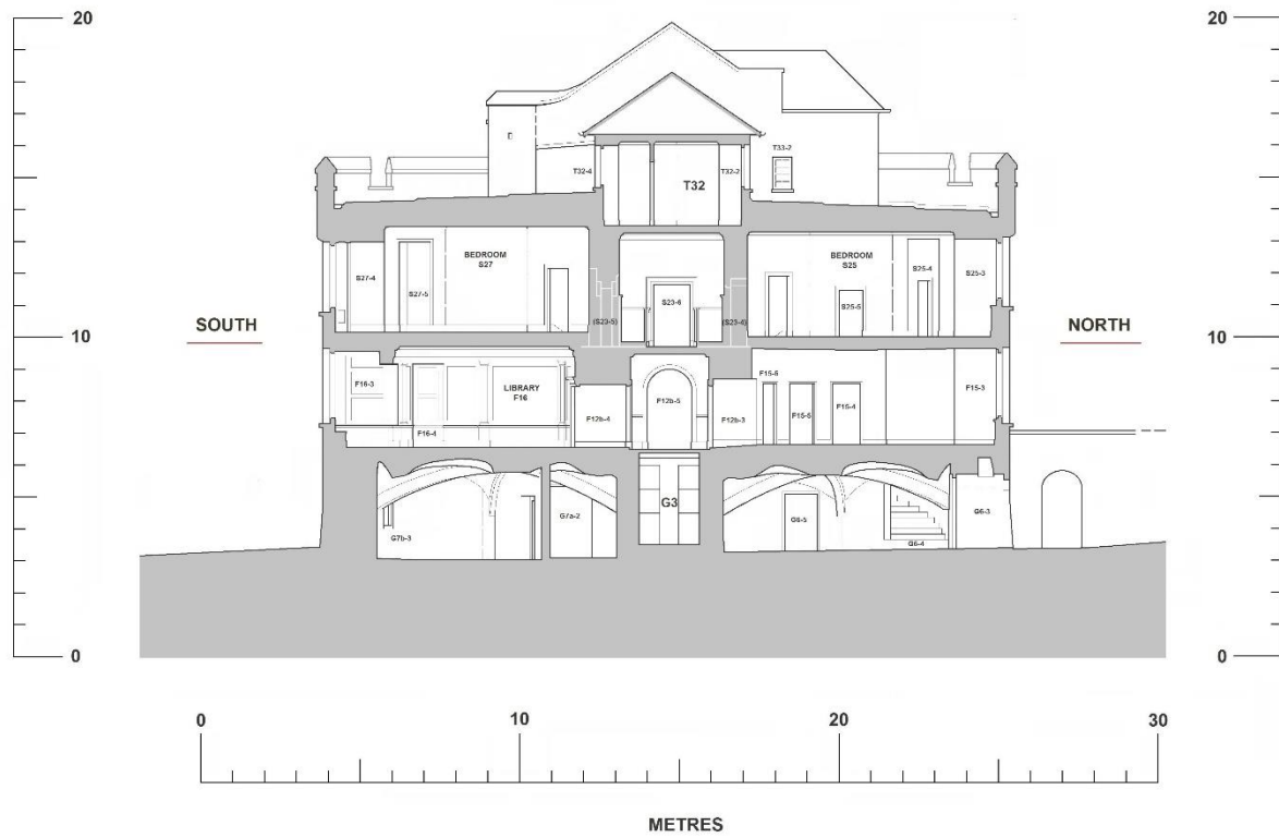
Fig. 178b: Transverse section through Picton Castle east towers, facing west – conjectured medieval
